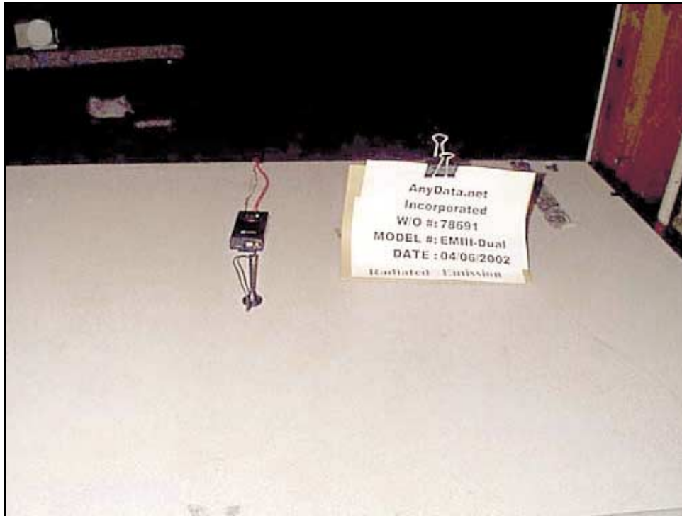
OATS Test Setup - Front View
