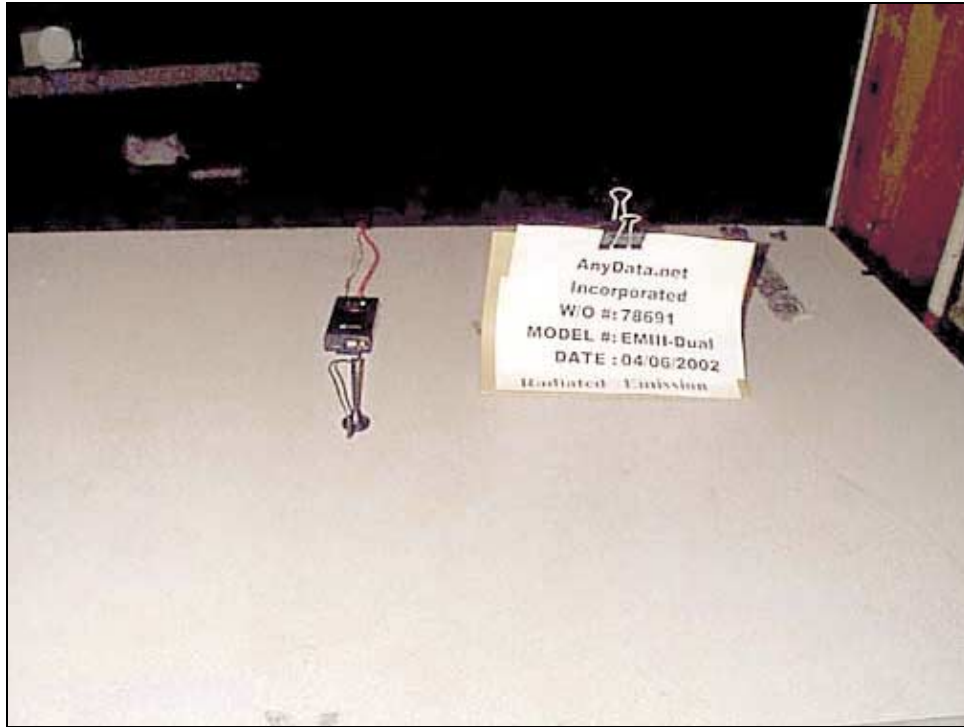
OATS Test Setup - Front View
