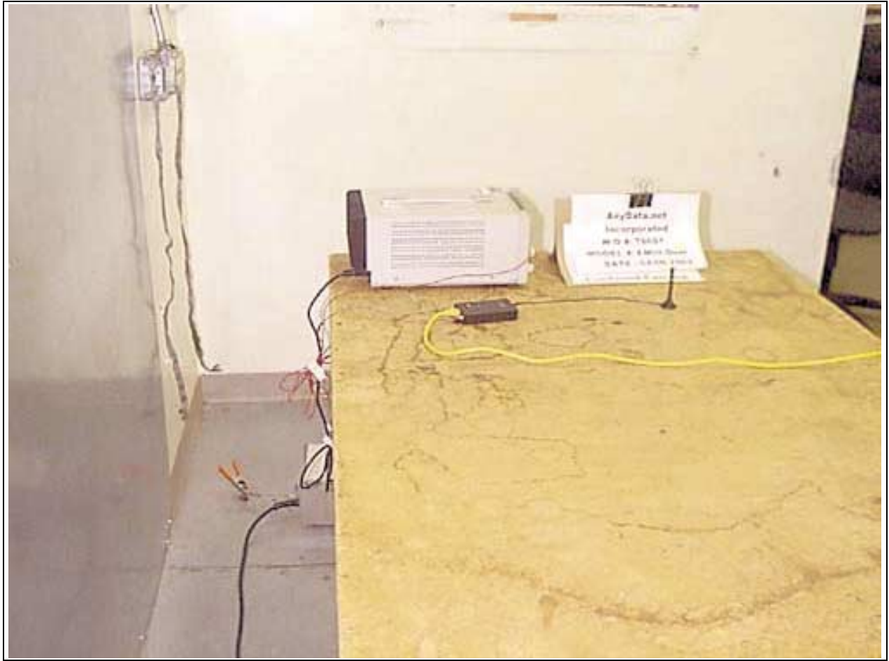
Mains Conducted Emissions - Side View
