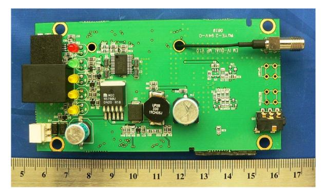
EUT – Radio Module Detail View (RF Shielding Removed)
