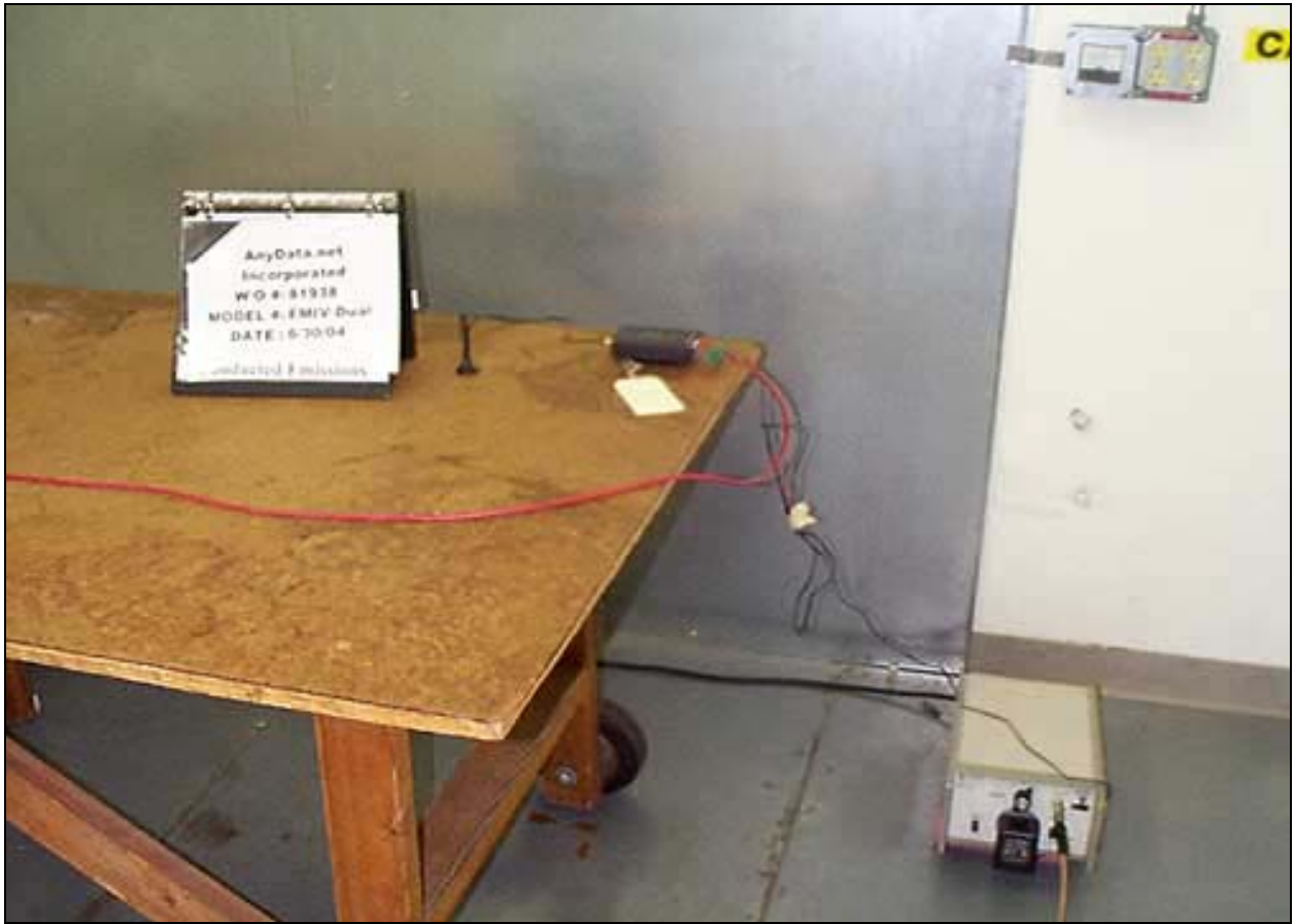
Mains Conducted Emissions - Front View
