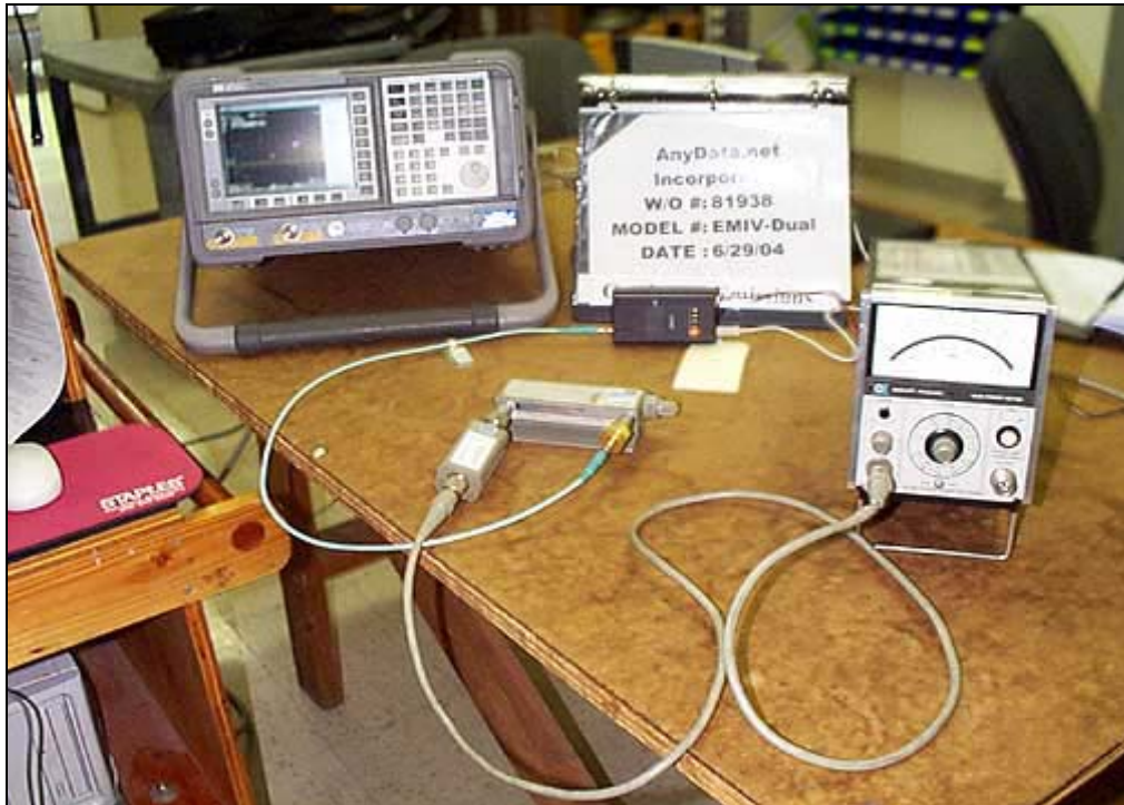
PHOTOGRAPH SHOWING DIRECT CONNECT TEST SETUP
