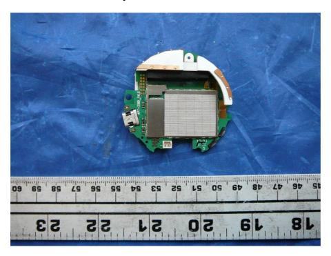
14.10 EUT Internal – RF Board Assembly Bottom (With RF Sheilding) View
