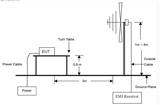
The diagram below shows the test setup that is utilized to make the measurements for emission from 1 GHz to 24 @ Emissions.
