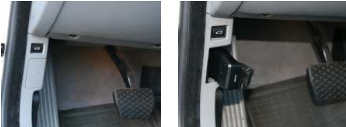
Figure 4.1: Installation of ACT613 in vehicle
