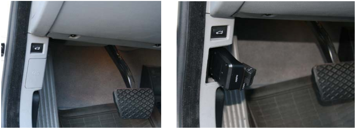
Figure4.1: Installation of ACT200-D in vehicle
