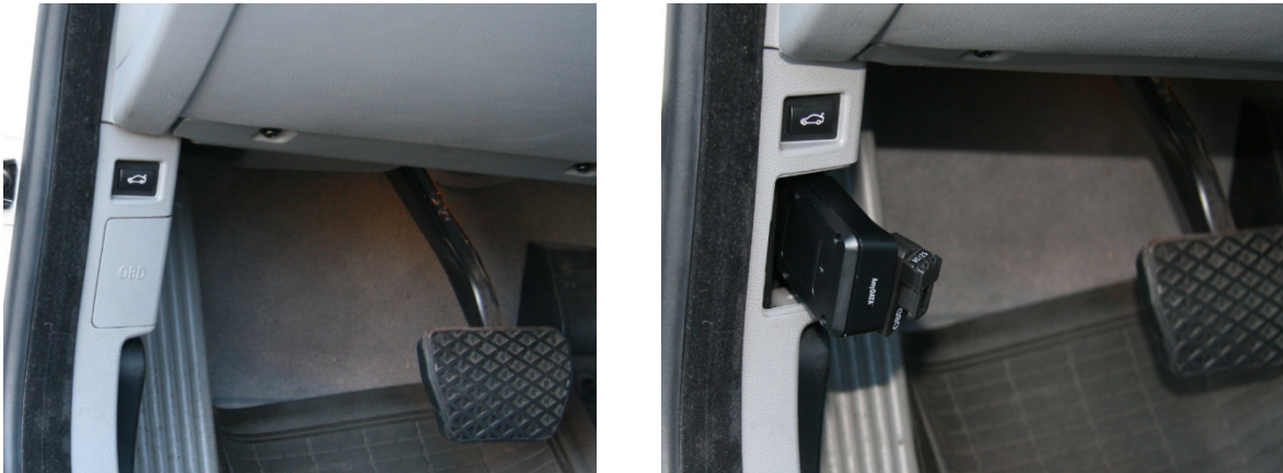
Figure 4.1: Installation of ACT10 in vehicle
