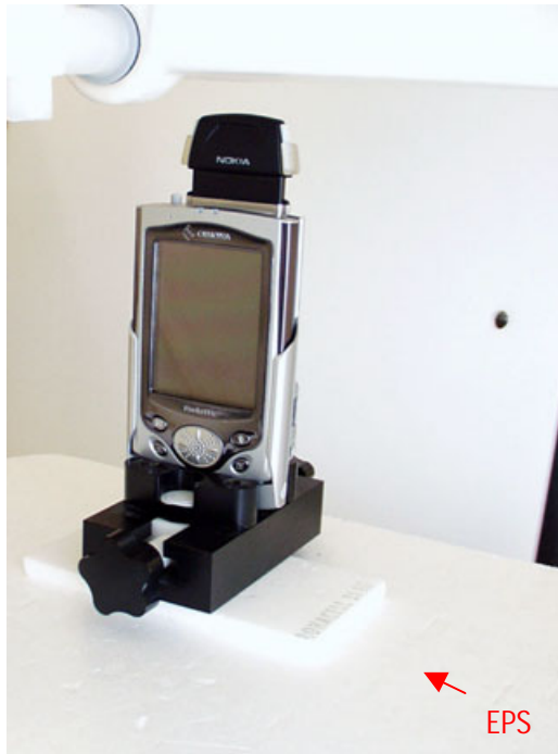
Pocket PC Casio Cassiopeia, all the pocket PCs were positioned similarly for testing the tip of P4JDTE-3 with separation distance 15mm.
