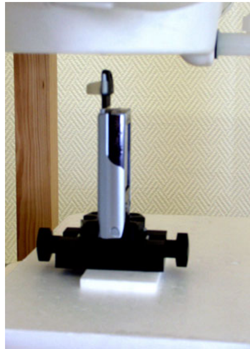
Pocket PC Casio Cassiopeia, all the pocket PCs were positioned similarly for testing the tip of P4JDTE-3 with separation distance 15mm.
