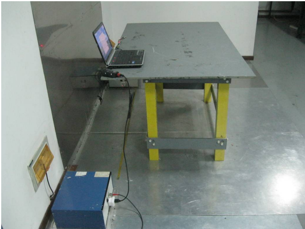
Conducted Emissions Setup Side View
