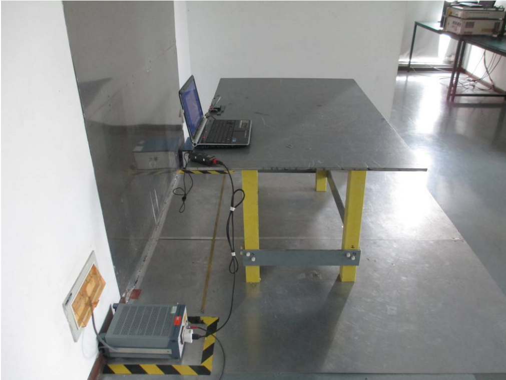
Conducted Emissions Test Setup Side View
