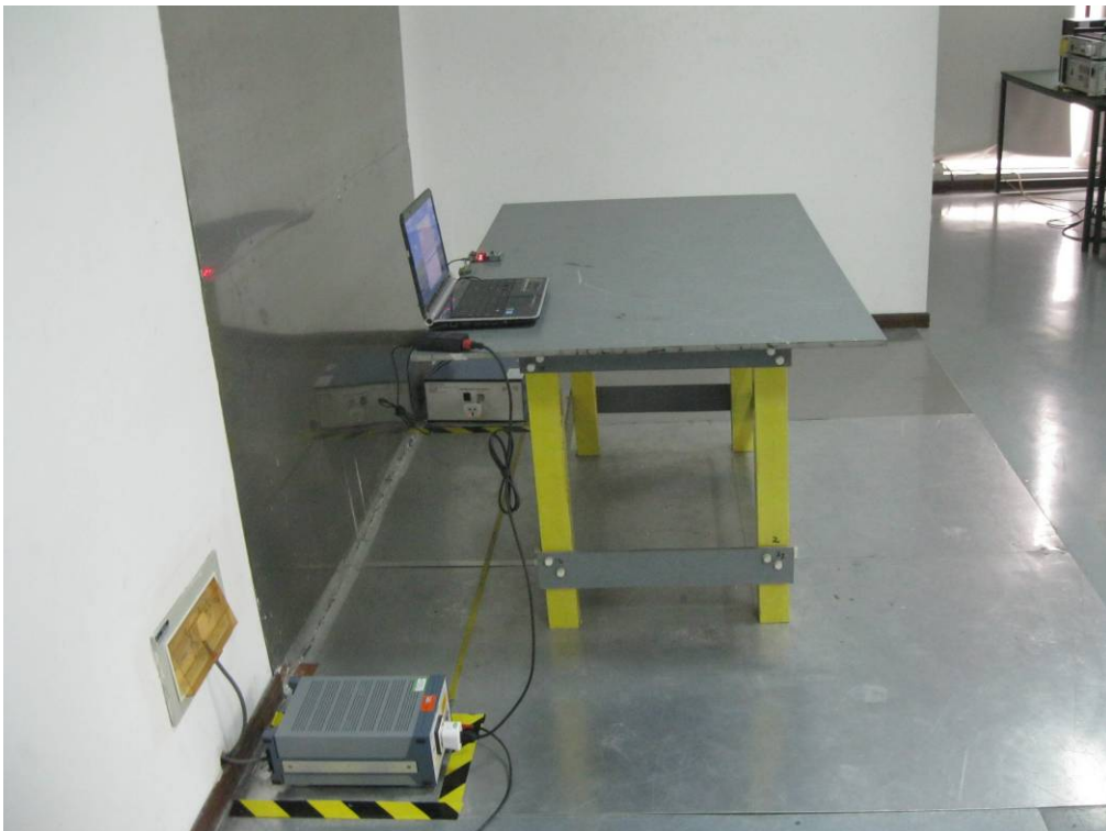
Conducted Emissions Test Setup Side View
