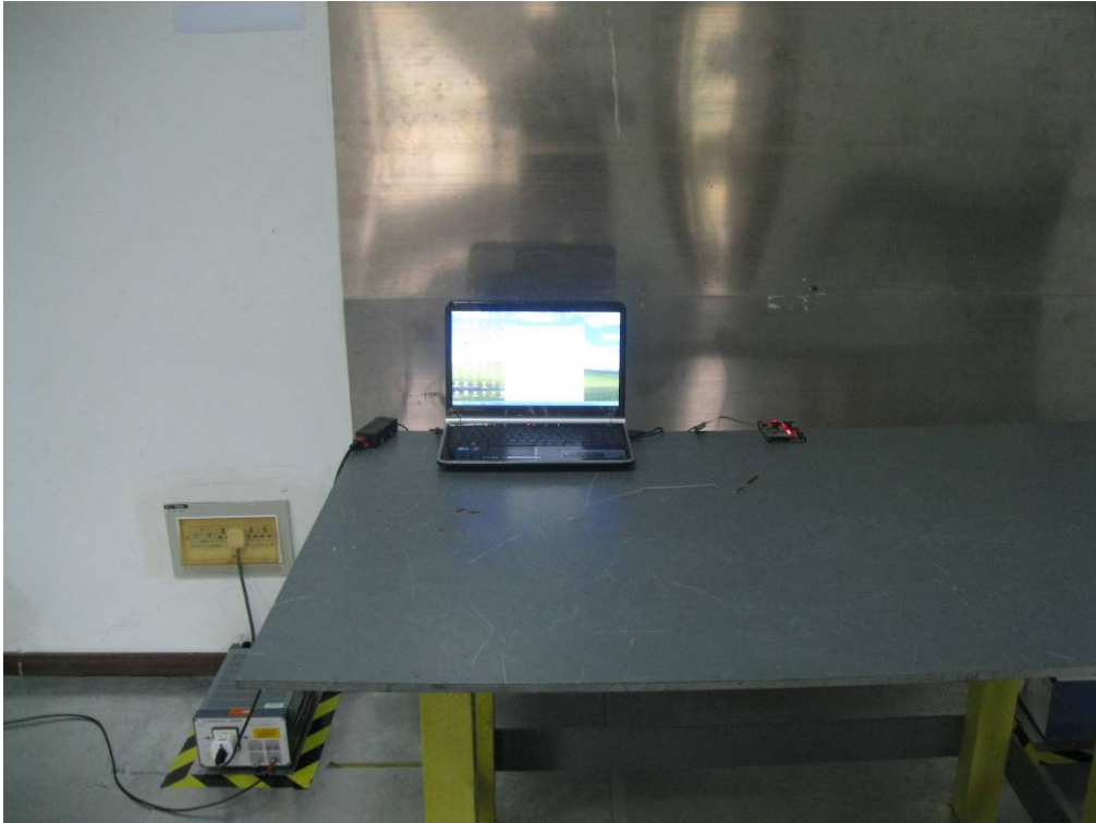
Conducted Emissions Test Setup Front View
