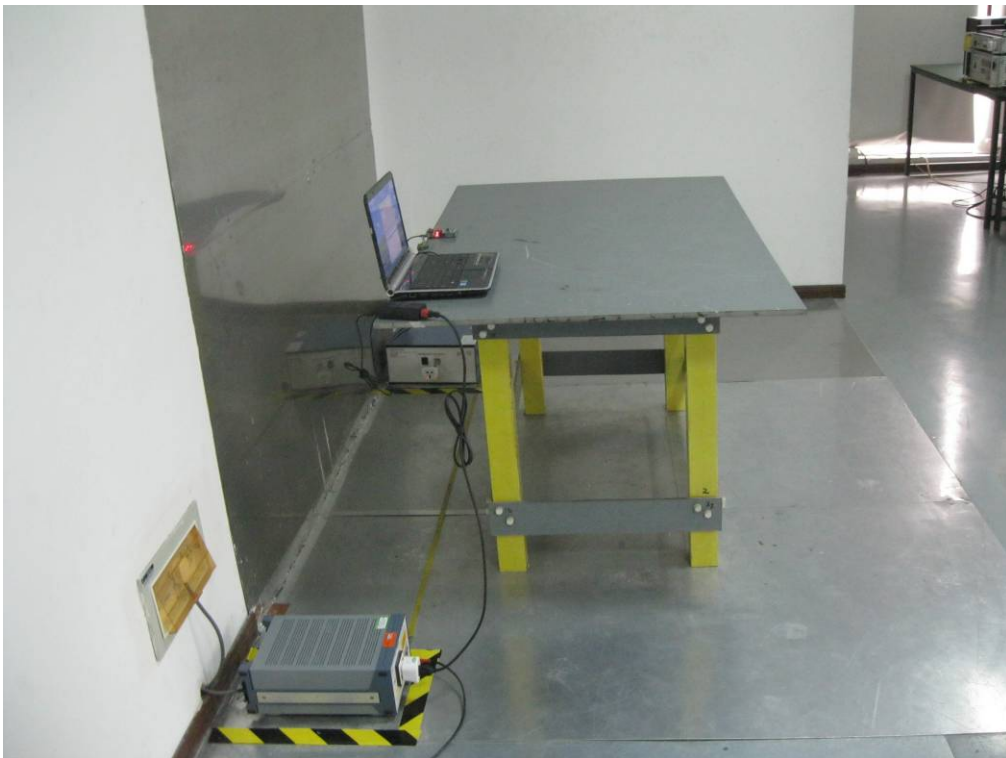
Conducted Emissions Test Setup Side View
