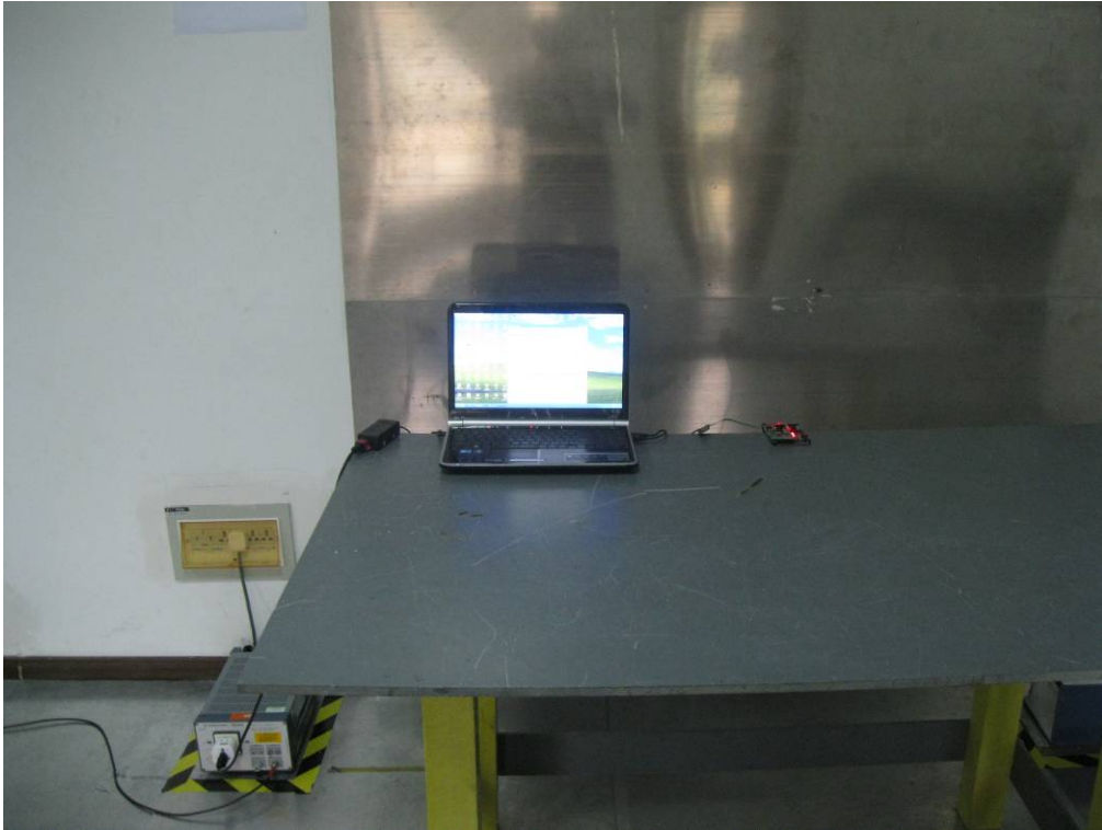
Conducted Emissions Test Setup Front View
