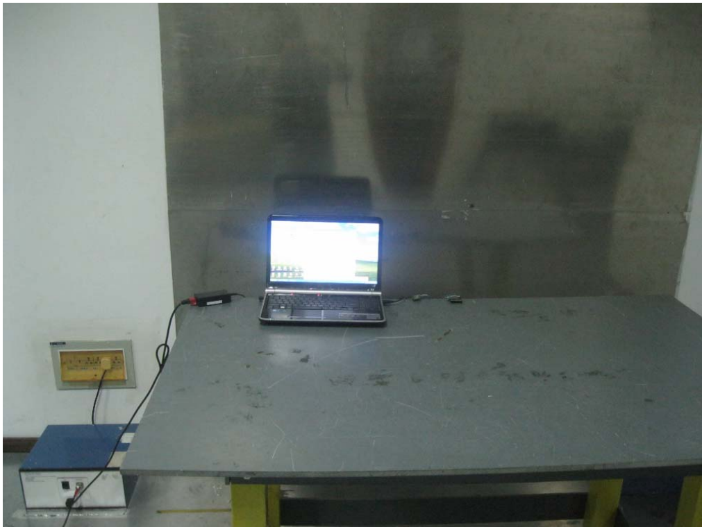
Conducted Emissions Test Setup - Front View
