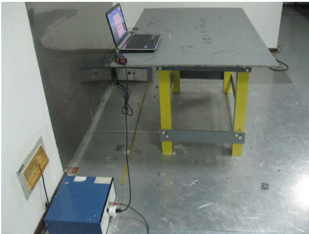
Conducted Emissions Test Setup - Side View
