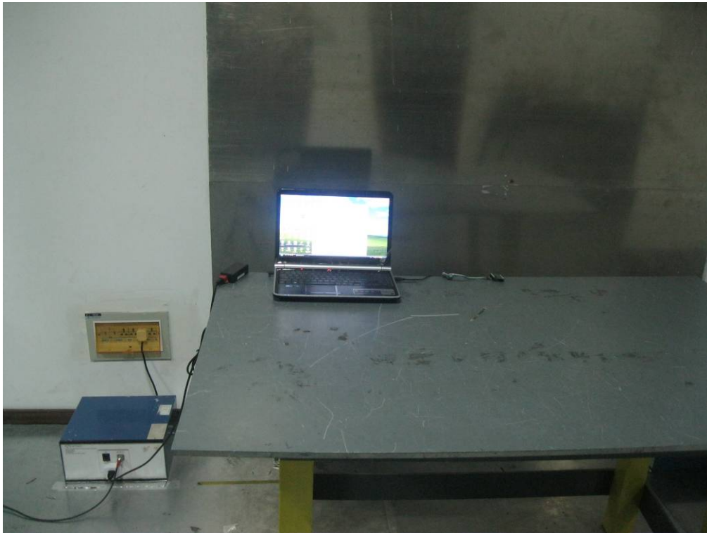
Conducted Emissions Setup Front View
