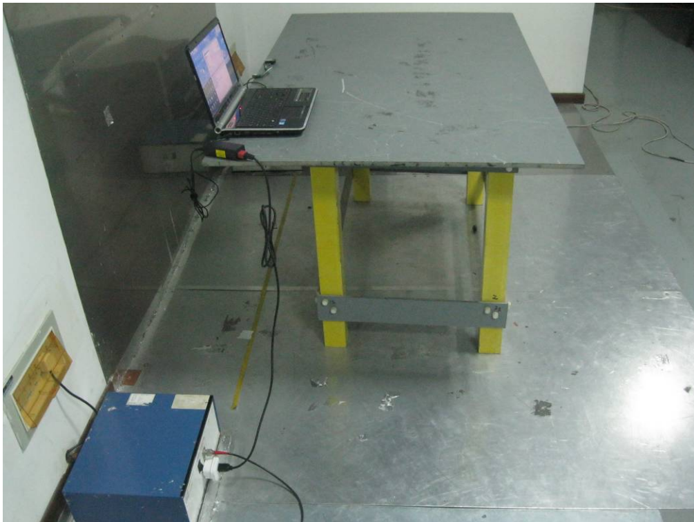
Conducted Emissions Setup Side View
