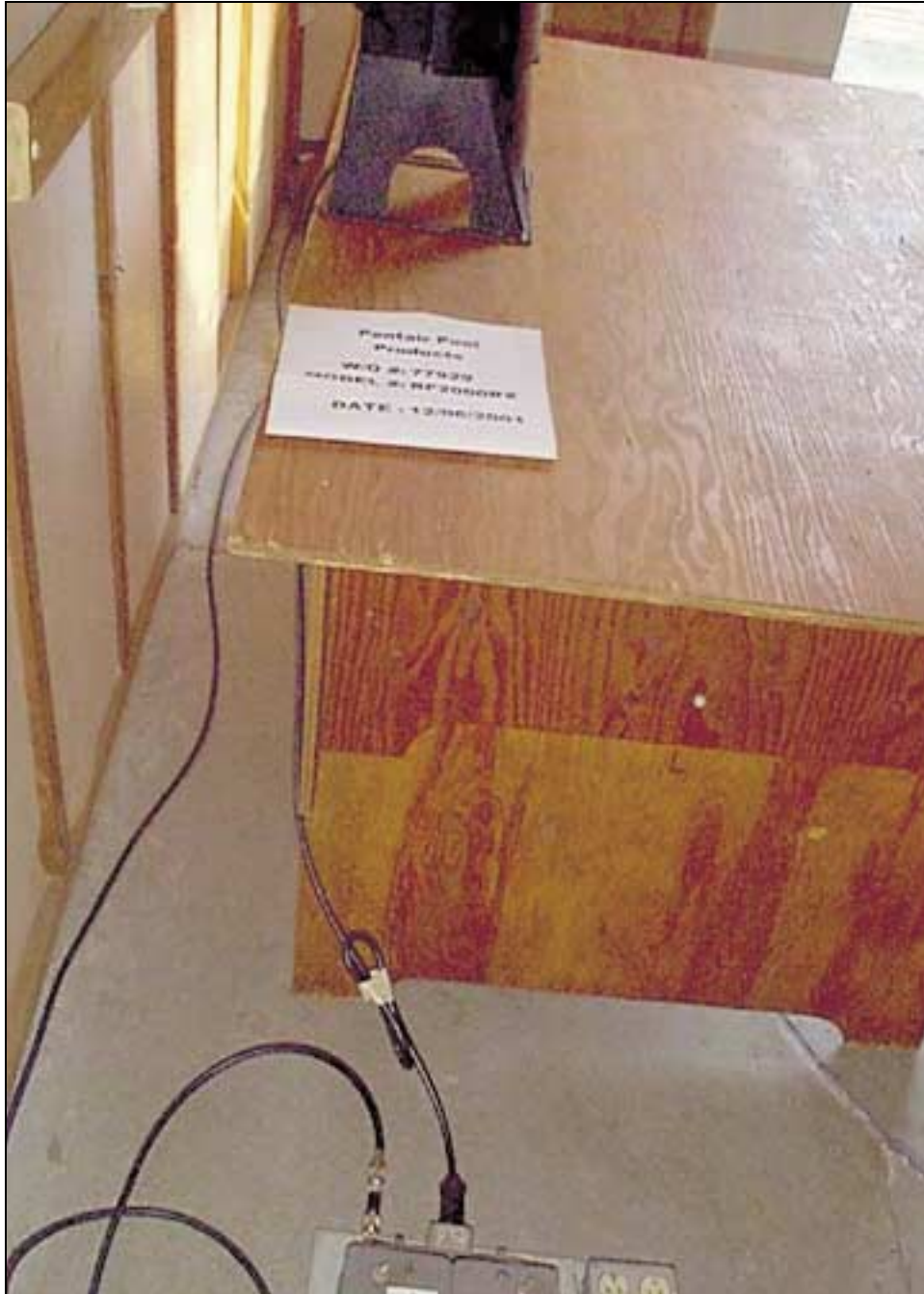
Mains Conducted Emissions - Side View of Receiver
