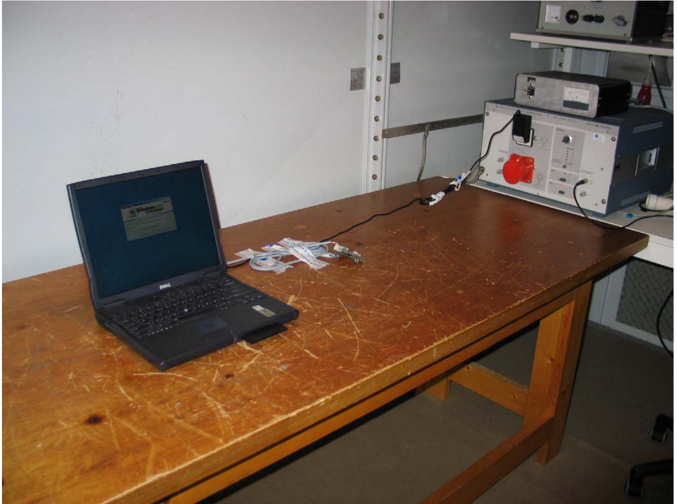
Photo 4 conducted emission measurement set up
