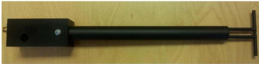
Figure 1 – MVG COMOSAR Validation Dipole
