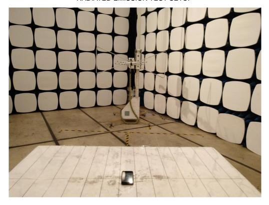
RADIATED EMISSION ABOVE 1G TEST SETUP
