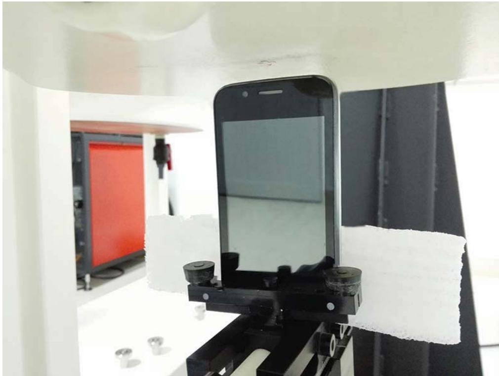
10mm Hotspot Mode Top Edge Setup Photo
