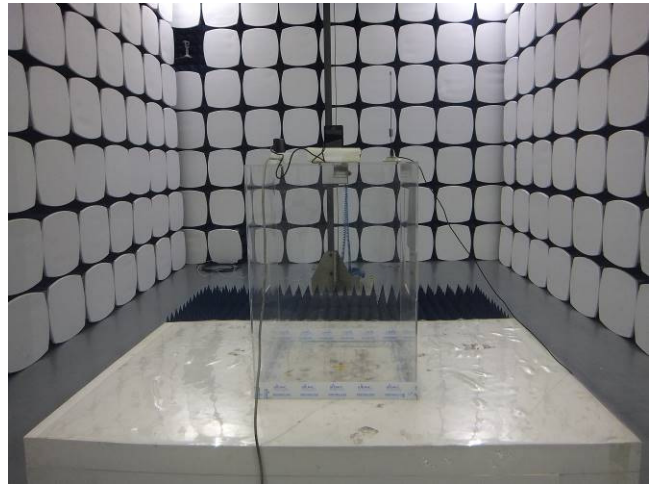
Radiated Spurious Emissions Test Setup Above 1GHz
