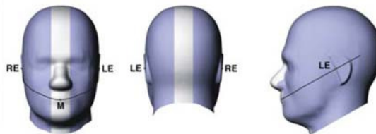
Figure 6.2 Front, back and side view of SAM
