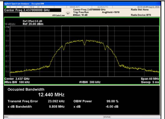
802.11b 6dB Bandwidth - Mid CH 2437
