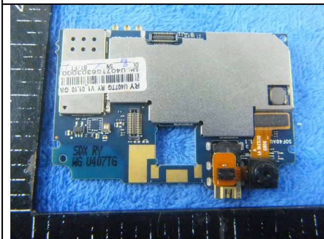
Mainboard with Shielding - Front View
