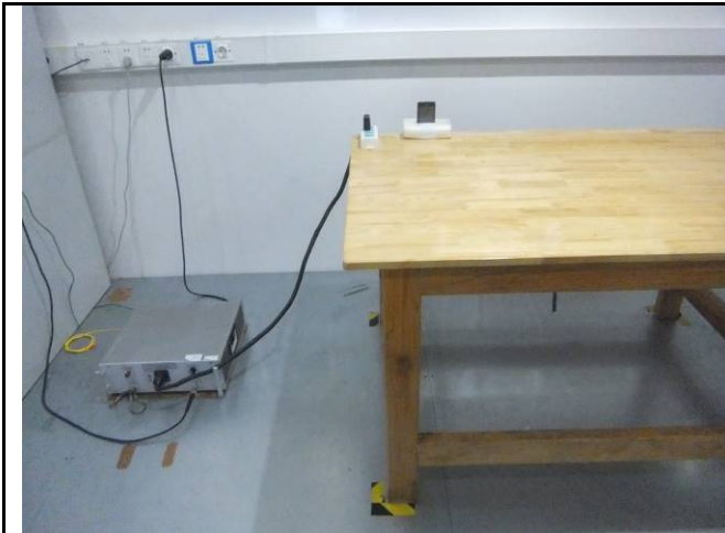
Conducted Emissions Test Setup Front View
