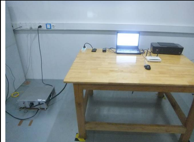
Conducted Emissions Test Setup – Front View
