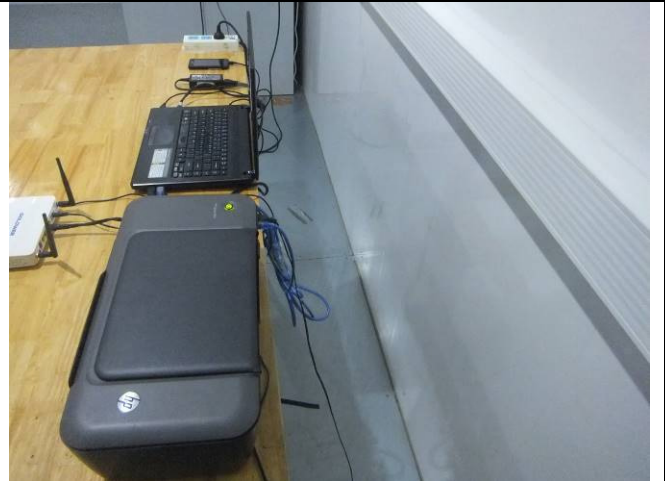
Conducted Emissions Test Setup – Side View
