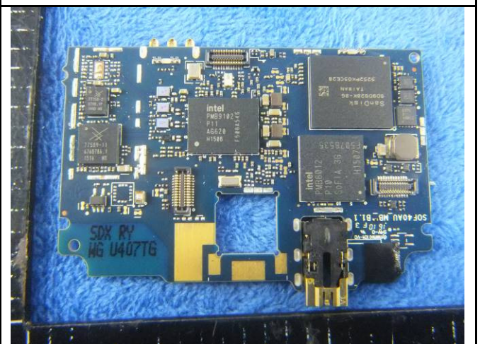
Mainboard without Shielding - Front View
