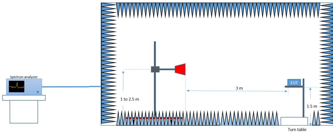
*Radiated Setup > 18GHz*
