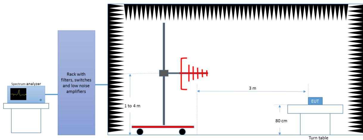
*Radiated Setup 1GHz - 18GHz*
