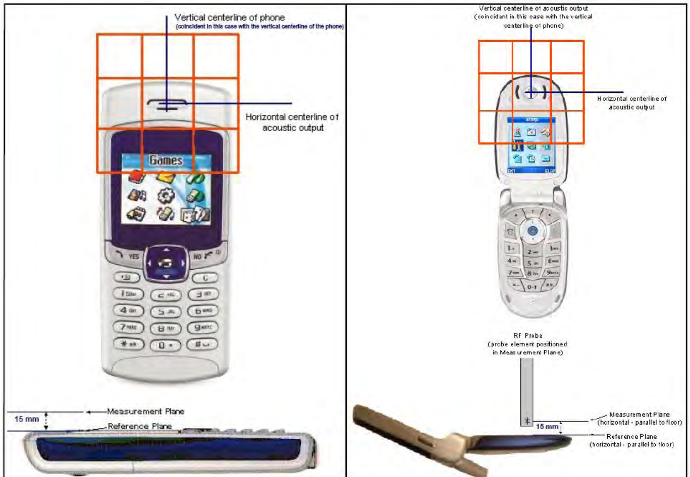
Fig-3.5 EUT Reference and Plane
