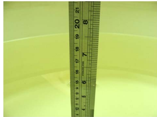
Fig 6.2 Photo of Liquid Height for Body SAR
