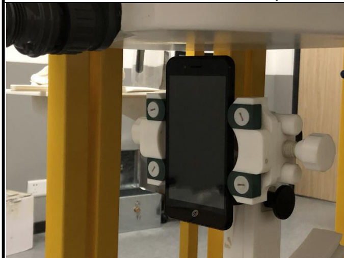
Top Side of EUT with 1.0 cm Gap
