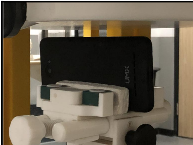
Left Side of EUT with 1.0 cm Gap
