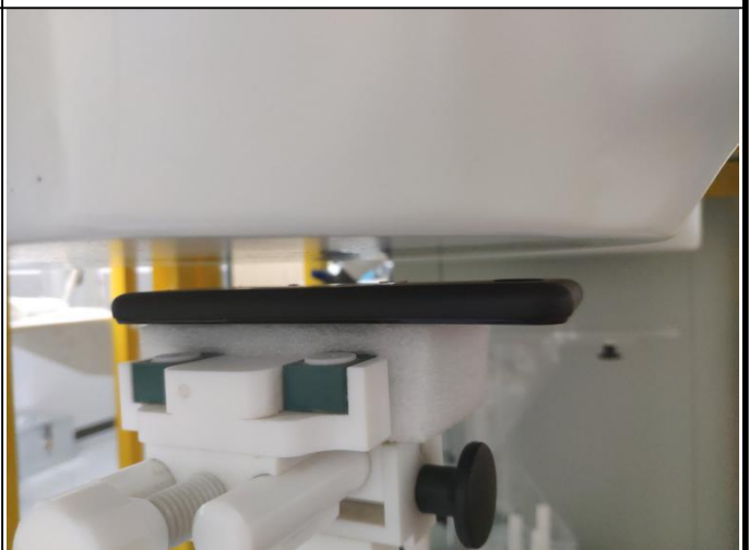
Rear Face of EUT with 1.0 cm Gap
