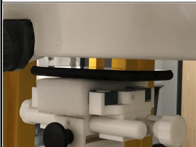
Front Face of EUT with 1.0 cm Gap
