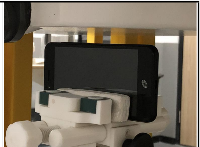
Right Side of EUT with 1.0 cm Gap
