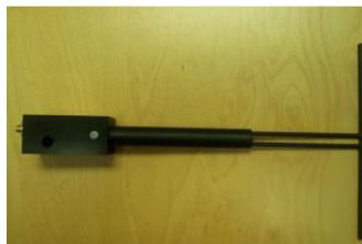
Figure 1 – MVG COMOSAR Validation Dipole
