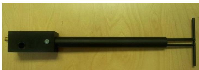
Figure 1 – MVG COMOSAR Validation Dipole
