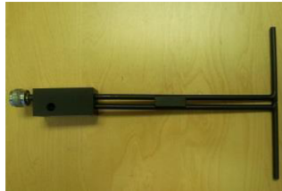
Figure 1 – MVG COMOSAR Validation Dipole
