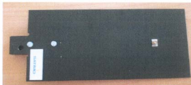
Figure 1 – Satimo COMOHAC Validation Dipole
