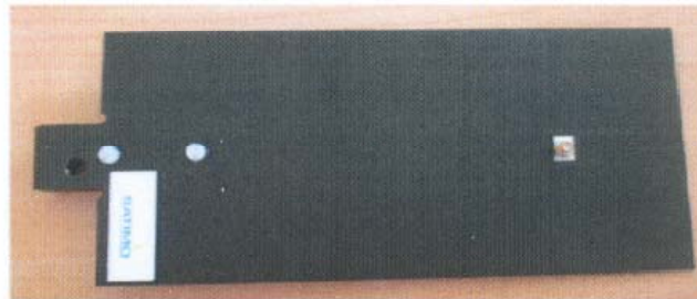
Figure 1 – Satimo COMOHAC Validation Dipole
