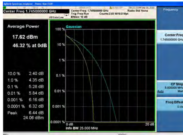
Band66 / 20MHz / Mid CH / 64QAM
