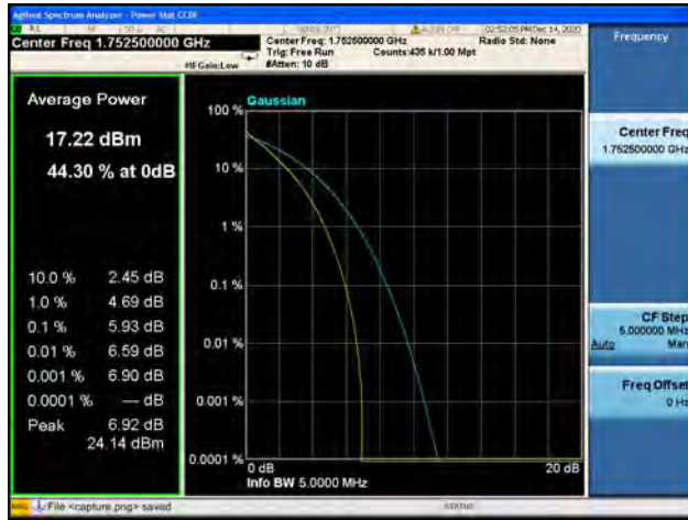
Band4 / 5MHz / High CH / 64QAM
