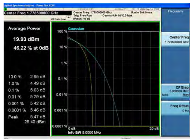
Band66 / 3MHz / High CH / 64QAM
