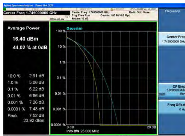
Band66 / 15MHz / Mid CH / 16QAM
