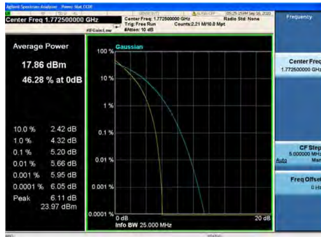
Band66 / 15MHz / High CH / 64QAM
