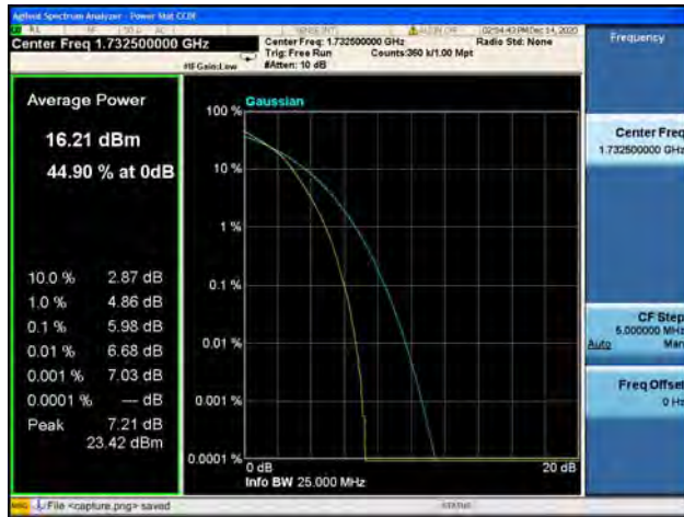
Band4 / 20MHz / High CH / 16QAM
