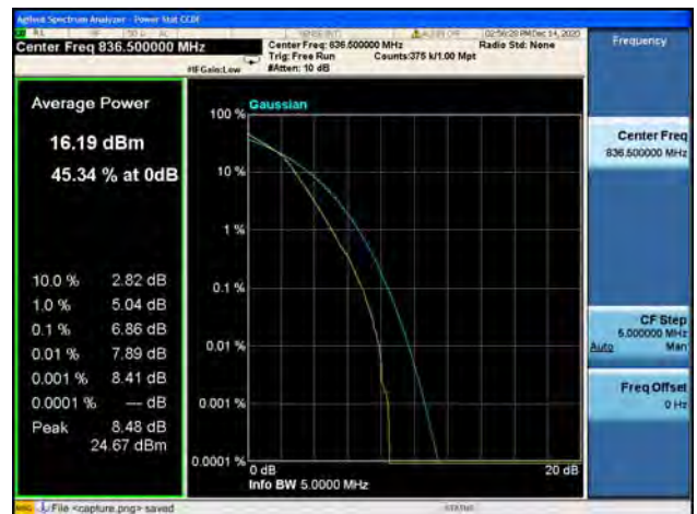
Band5 / 1.4MHz / Mid CH / 64QAM
