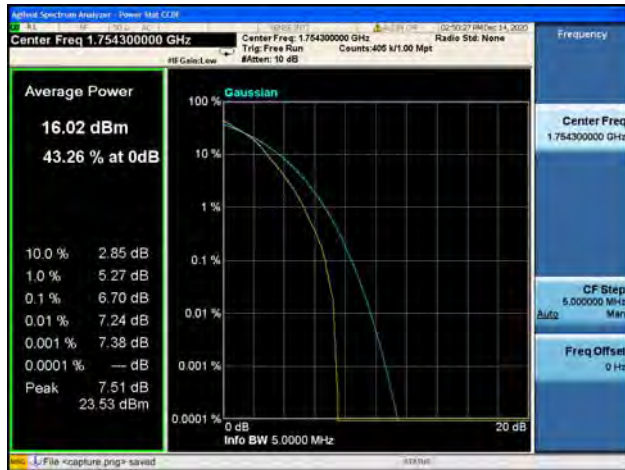
Band4 / 3MHz / Low CH / 16QAM
