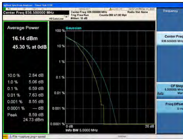
Band5 / 3MHz / High CH / 16QAM
