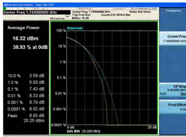
Band66 / 20MHz / High CH / 16QAM
