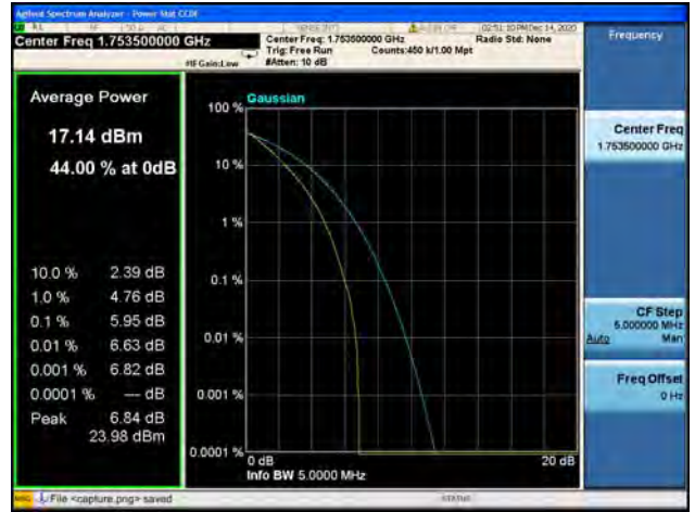
Band4 / 3MHz / High CH / 64QAM
