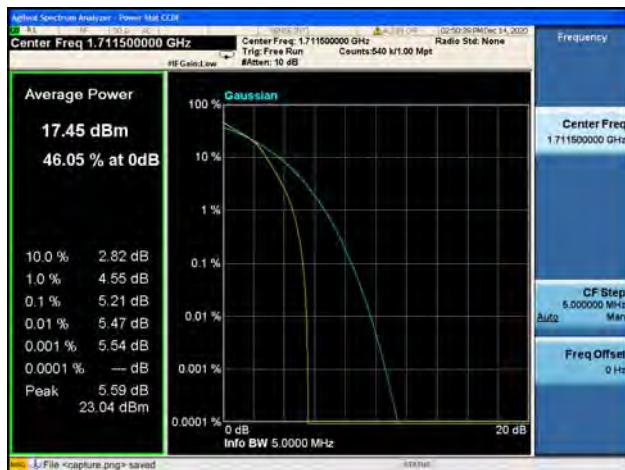
Band4 / 3MHz / Low CH / 16QAM
