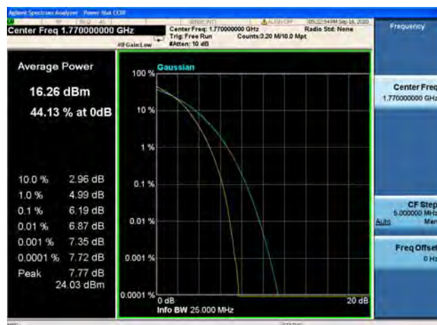
Band66 / 20MHz / High CH / 16QAM
