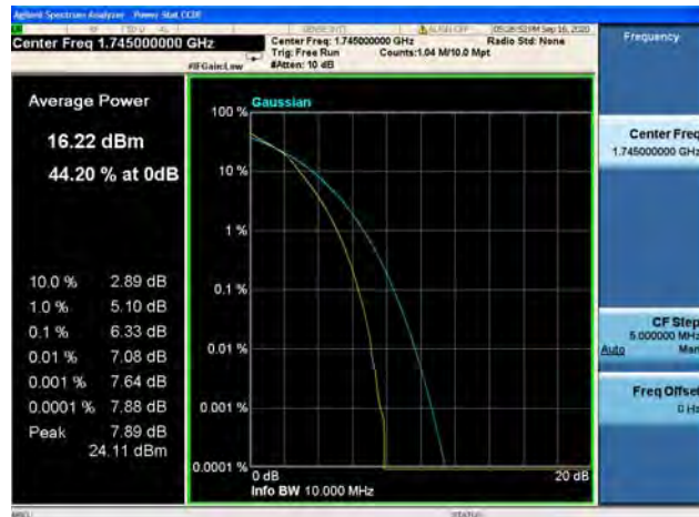
Band66 / 10MHz / Mid CH / 64QAM
