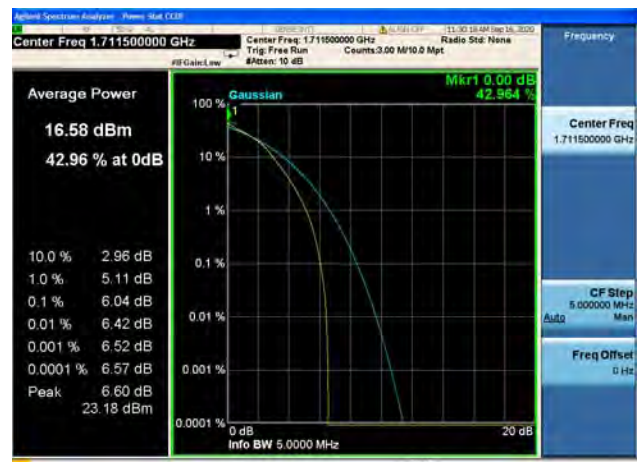
Band66 / 3MHz / Low CH / 64QAM
