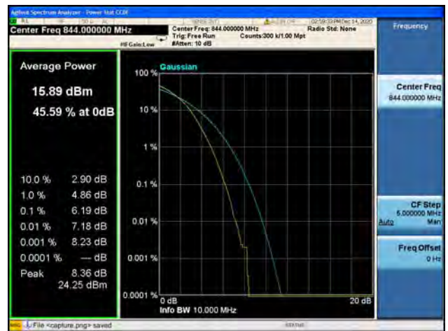
Band5 / 10MHz / High CH / 64QAM
