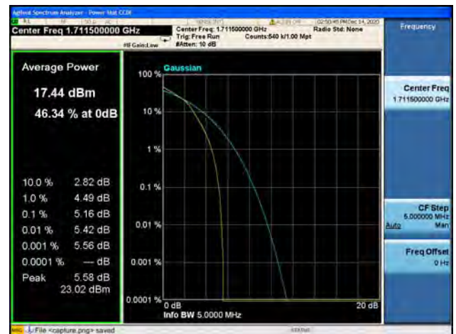
Band4 / 3MHz / Low CH / 64QAM
