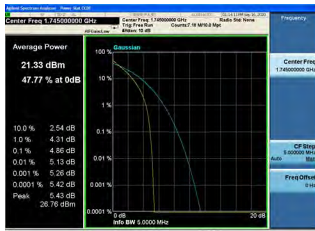
Band66 / 3MHz / High CH / 16QAM
