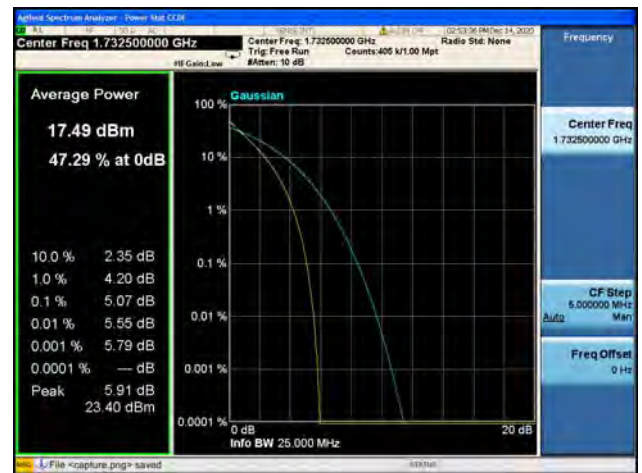
Band4 / 15MHz / Mid CH / 64QAM
