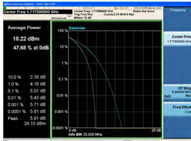
Band66 / 15MHz / Low CH / 64QAM
