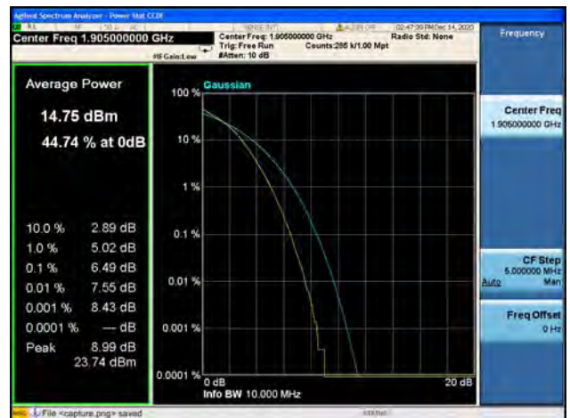
Band2 / 10MHz / High CH / 64QAM
