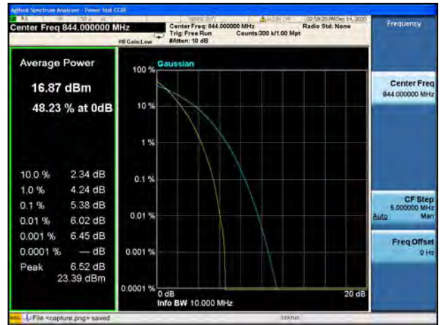
Band5 / 10MHz / High CH / 64QAM
