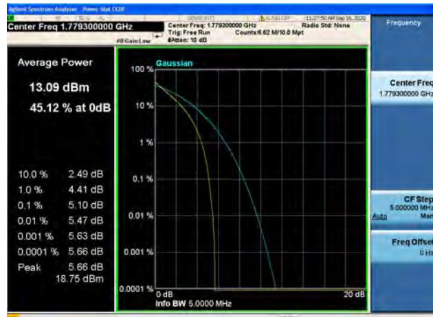
Band66 / 1.4MHz / High CH / 64QAM
