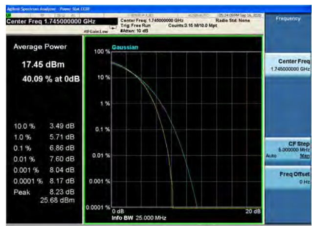
Band66 / 15MHz / Mid CH / 64QAM
