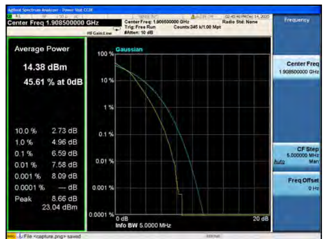
Band2 / 3MHz / High CH / 64QAM
