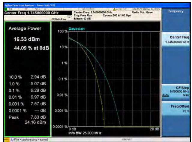
Band4 / 20MHz / High CH / 64QAM
