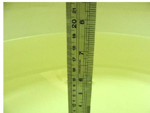
Fig 7.2 Photo of Liquid Height for Body SAR
