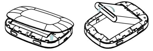
2. Place the battery cover over the battery compartment and press it downward until it clicks into place.
