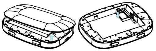
3. Insert the SIM card into the slot until it is fully inserted.
