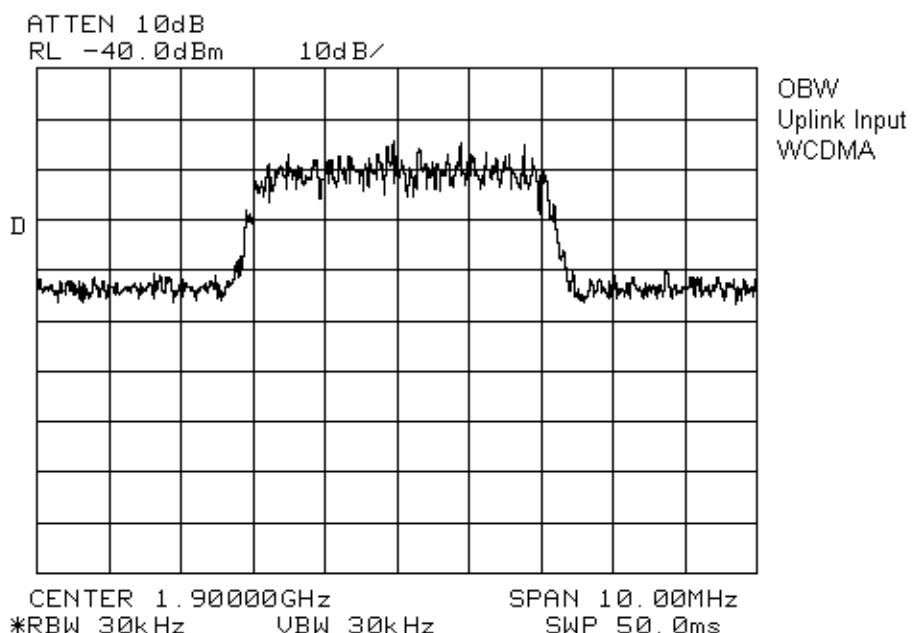
**Section 5. Spurious Emissions at Antenna Terminals****Para. No.: 2.1051****Test Performed By: Glen Westwell****Date of Test: 17 Sept 2004****Minimum Standard:** 24.238, -13dBm**Test Results:** Complies.
