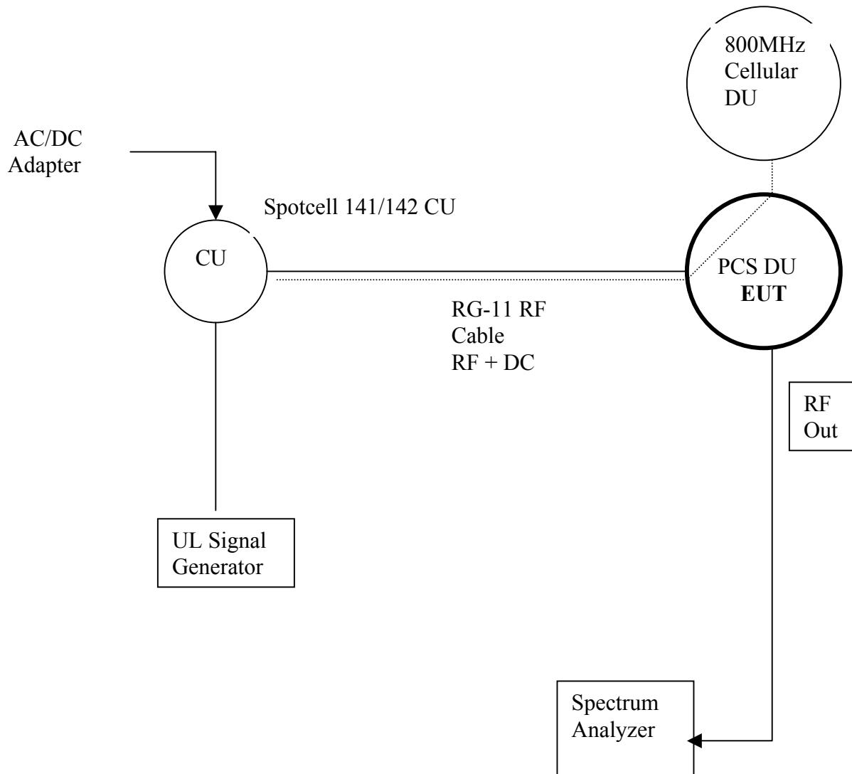
*EQUIPMENT: DU 1900 Full Band***Para. No. 2.1046 - R.F. Power Output**
