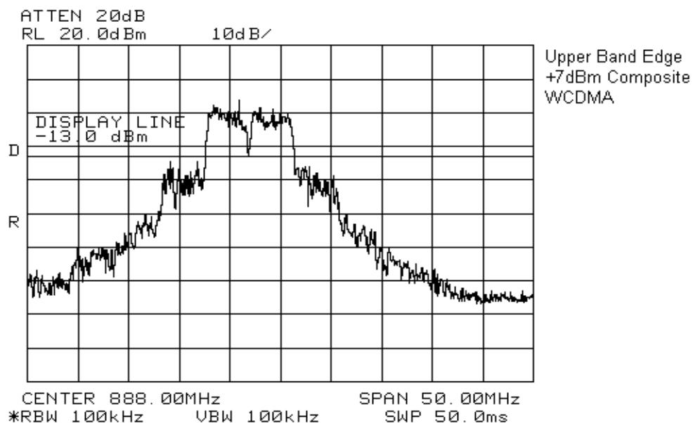
**Section 7. Field Strength of Spurious Emissions****Para. No.: 2.1053**
