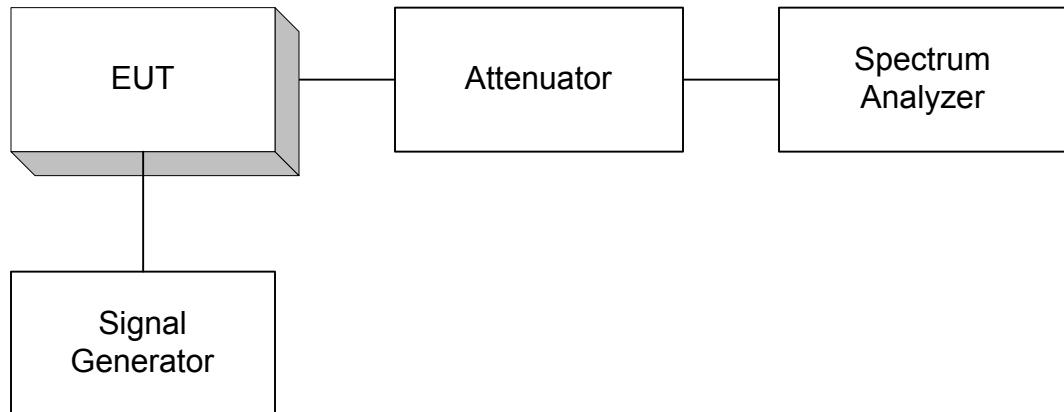
*EQUIPMENT: Spotcell 141/142, 111/112***Para. No. 2.1051 - Spurious Emissions at Antenna Terminals**
