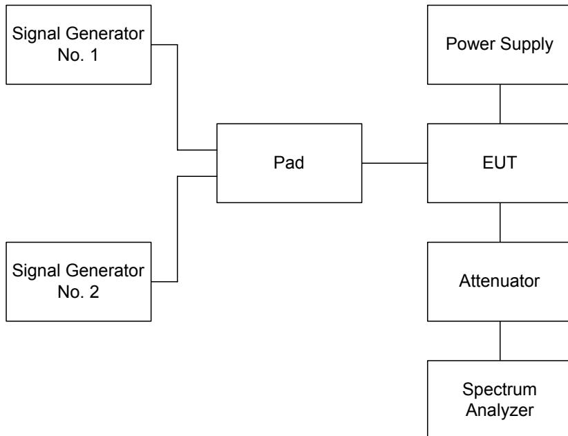
**Para. No. 2.1053 - Field Strength of Spurious Radiation****TIA/EIA 603**
