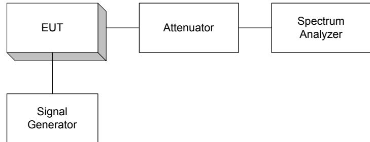
*EQUIPMENT: Spotcell 163, iDEN, DU***Para. No. 2.1051 - Spurious Emissions at Antenna Terminals**
