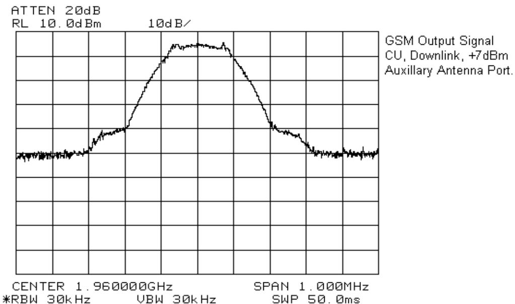
**Section 5. Spurious Emissions at Antenna Terminals****Para. No.: 2.1051**
