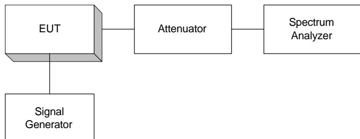
**Para. No. 2.1053 - Field Strength of Spurious Radiation****TIA/EIA 603**
