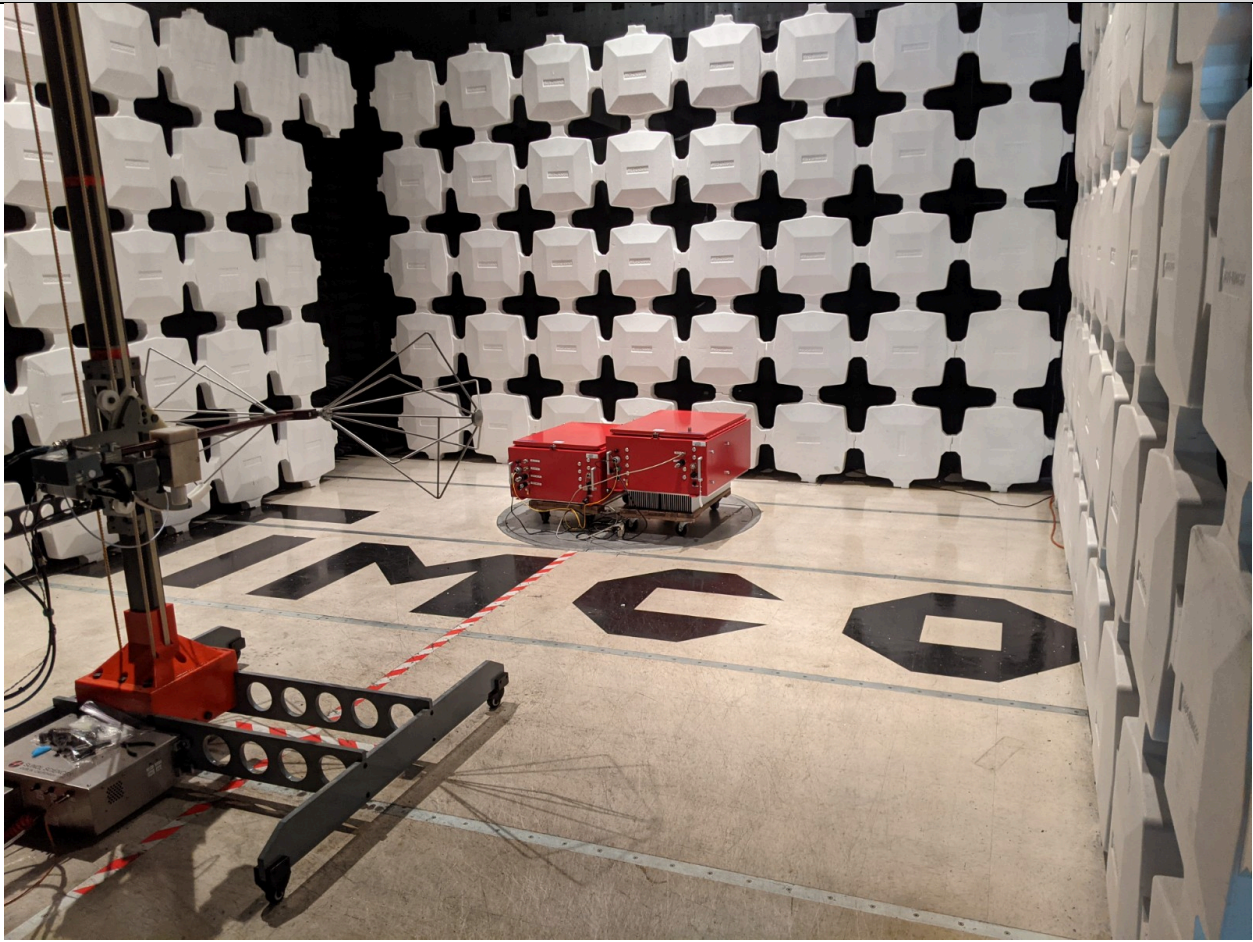
Radiated Testing, Below 1 GHz
