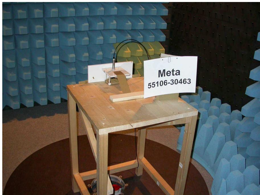
**Test setup for radiated emission measurement
