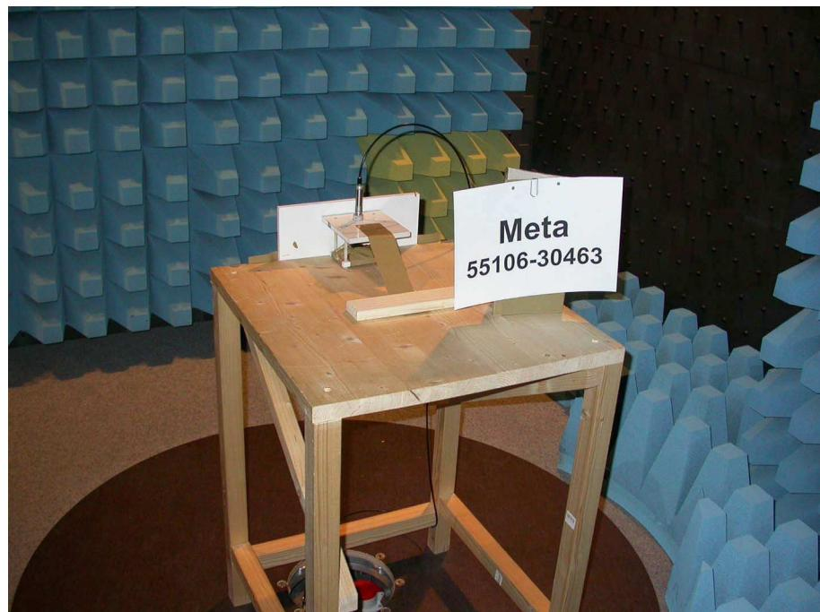
**Test setup for radiated emission measurement
