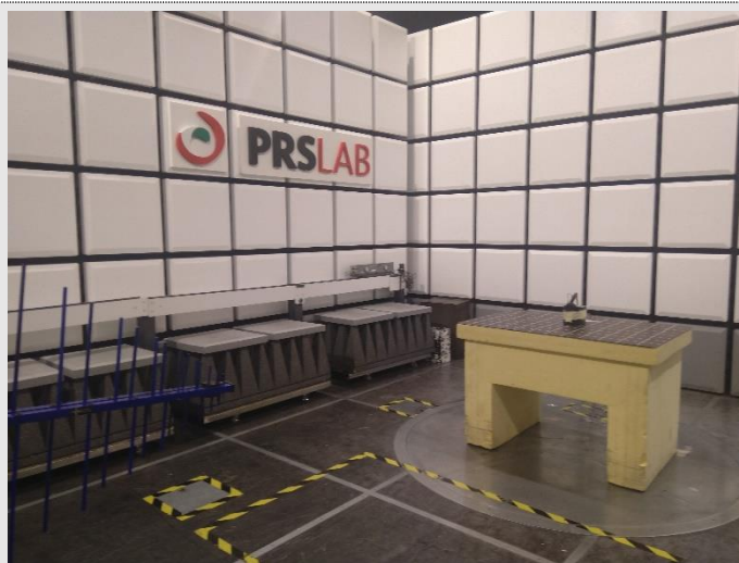
PHOTO N° 2 - RADIATED EMISSION TEST SETUP
