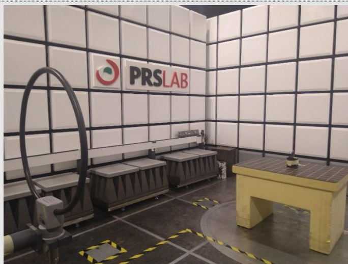
PHOTO N° 2 - RADIATED EMISSION TEST SETUP
