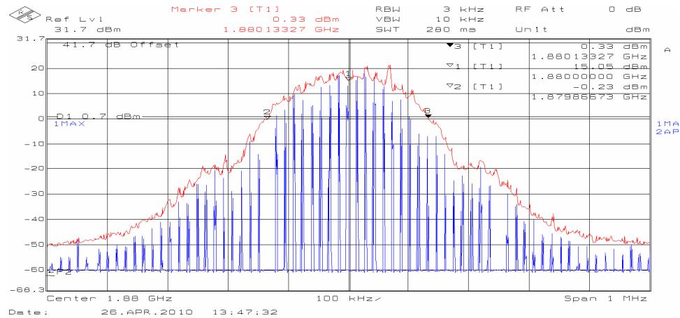
Display line 1: 1879.86673, Display line 2: 1880.13327 Bandwidth: 266.5kHz
