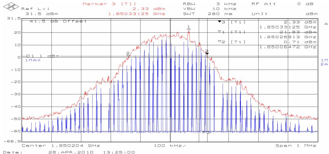
Display line 1: 1850.06472, Display line 2: 1850.33125 Bandwidth: 266.5 kHz
