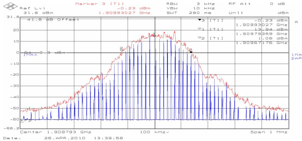
Display line 1: 1909.67176, Display line 2: 1909.93027 Bandwidth: 258.5 kHz
