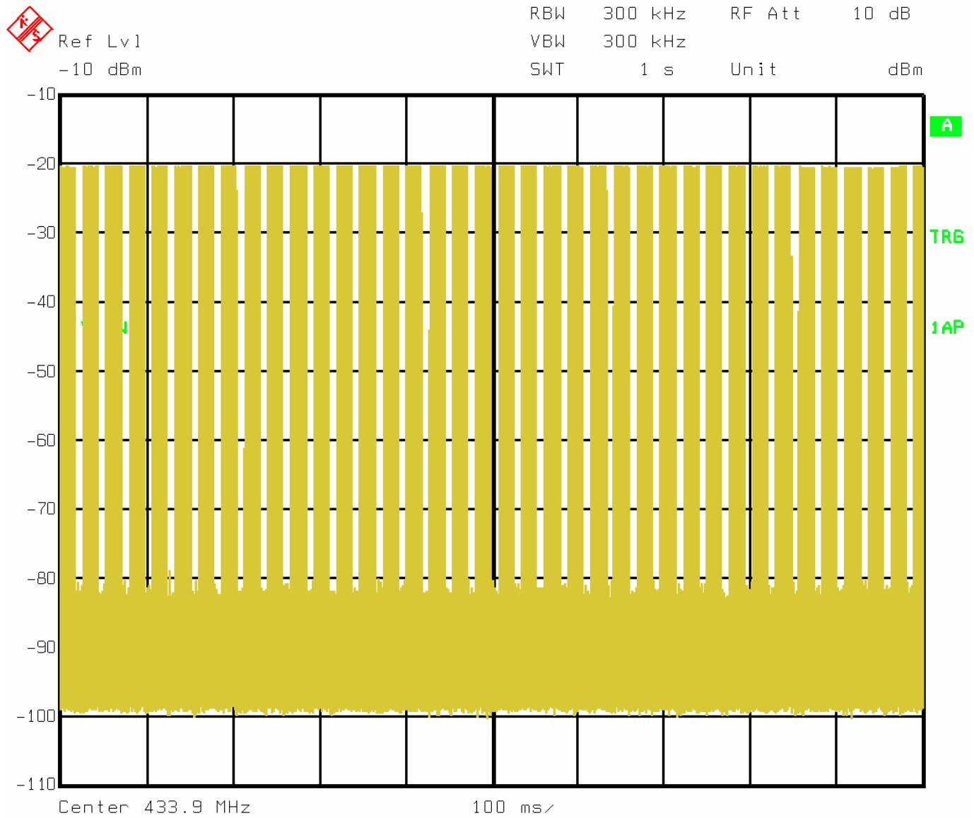
17 ms x 38 pulses in any 1000 ms → 646 ms TXon in any 1000 ms      →      64.6 ms TXon in any 100 ms
