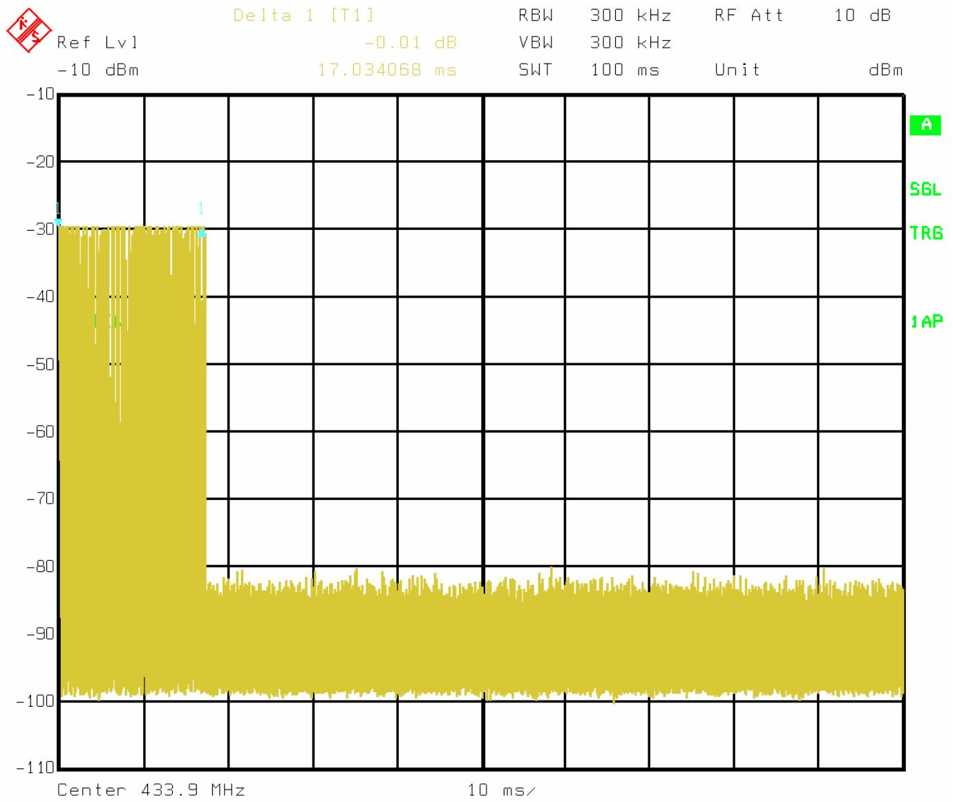
Correction factor  $20 \log (17. \text{ ms}/100 \text{ ms}) = -15.4 \text{ dB}$ .
