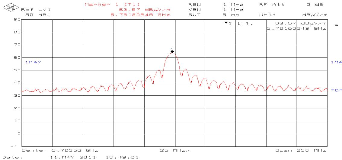
RBW of 1 MHz is less than the main lobe width. Therefore these measurements must be made using "Pulsed RF Agilent 150-2" test method with the spectrum analyzer configured for pulse spectrum. When the bandwidth (RBW) equals 1/2 of the main lobe width the displayed amplitude is practically the peak amplitude of the signal.
