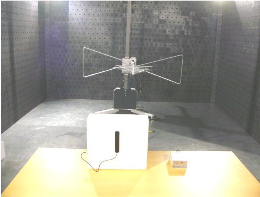
Radiated emission test view
