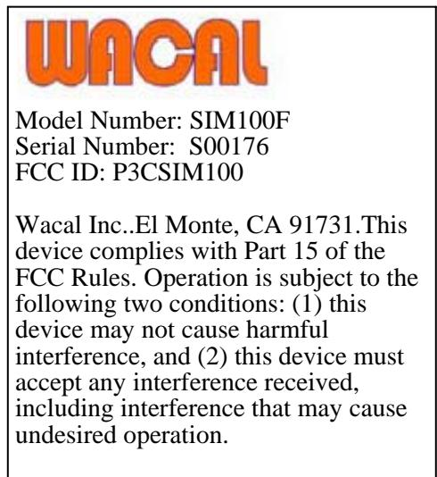
Specifications: Text is black or white in color and is left justified. Labels are silk-screened and shall be "permanently affixed" at a conspicuous location on the EUT.
