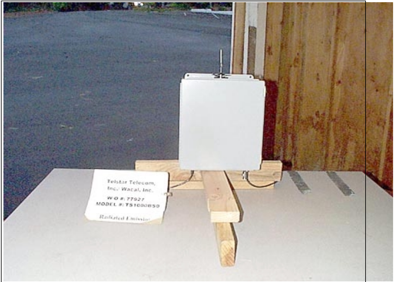
Radiated Emissions - Front View of Base Station
