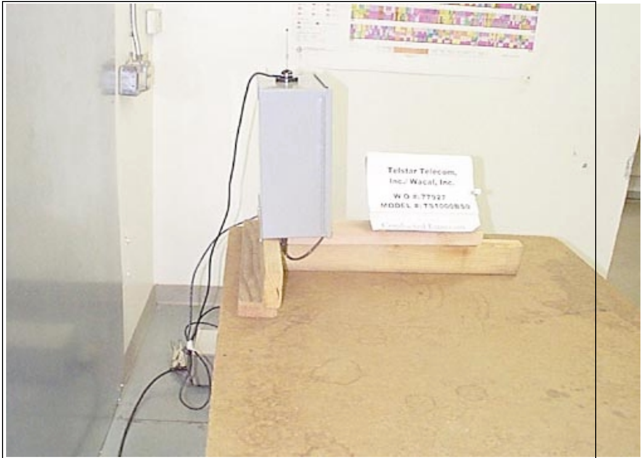
Mains Conducted Emissions - Side View of Base Station
